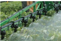
Wet Boom Plumbing
