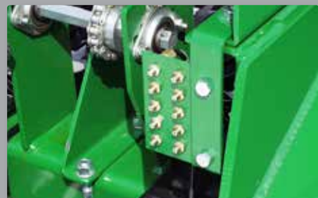
GREASE BANK - Lets you service all the coulters pivot components from two locations.
