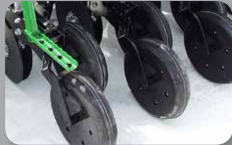
STAGGERED OPENERS - 10 3/4" of stagger between rows provides unobstructed residue flow through the machine.
