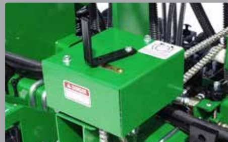
4-SPEED GEARBOX - Metering rate can be changed quickly and conveniently from a single location.
