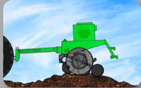
END WHEEL DESIGN - Keeps all ground-working components in line with the end wheels, preventing sideloading.
