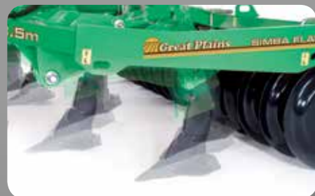
HYDRAULIC RESET SYSTEM - Flatliner Hydraulic Reset - The tines can cope with high stone content soils and varying field conditions. Each tine is hydraulic, offering a fast responsive trip and re-setting action on the move. Auto resetting pressure is adjustable. The hydraulic system is fully pressurised for minimal maintenance and wear.
