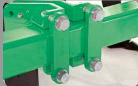
ADJUSTABLE TINE CLAMPS - Flatliner 500 - Adjustable tine clamps offer increased flexibility.
