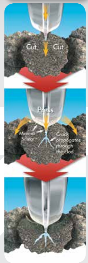
Clods are cut and fissures propagate through a result of the DD action, Broken or cracked clods are left in an ideal state for further weathering
