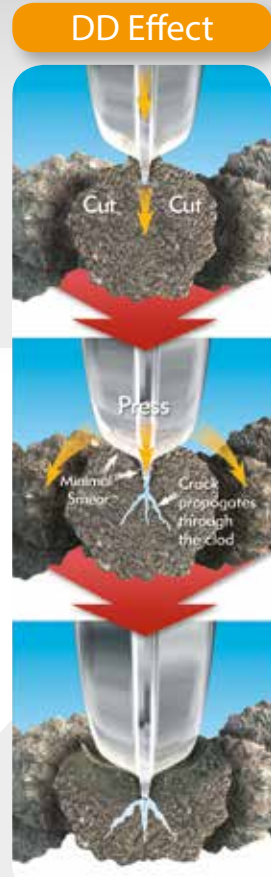
Clods are cut and fissures propagate through a result of the DD action, Broken or cracked clods are left in an ideal state for further weathering
