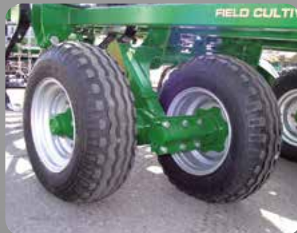
WALKING AXLE - 6 stub-axle hubs give improved strength and durability.
