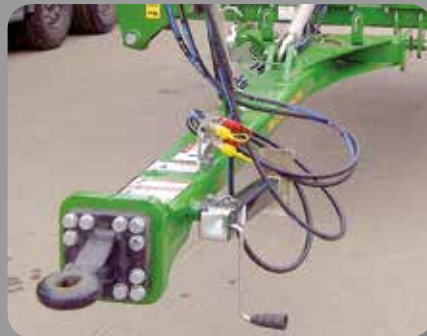
HITCH - Scharmüller ISO flange plate with fixing bolts.
