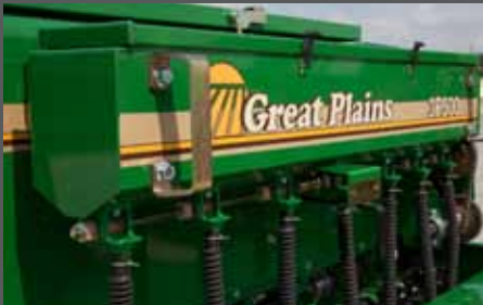
SMALL SEEDS ATTACHMENT - Utilizes a smaller version of the fluted feed cup to accurately meter tiny seeds like alfalfa and wildflowers.
