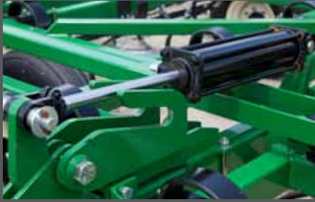
FOLDING SYSTEM - Improved fold system with heavier hinges on both inside and outside wings.
