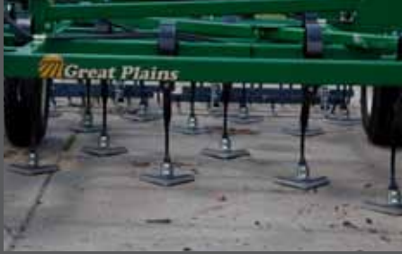
SHANK IMPROVEMENT - Improved shank spacing around tires and throughout the machine with no shanks closer than 28" on entire implement.
