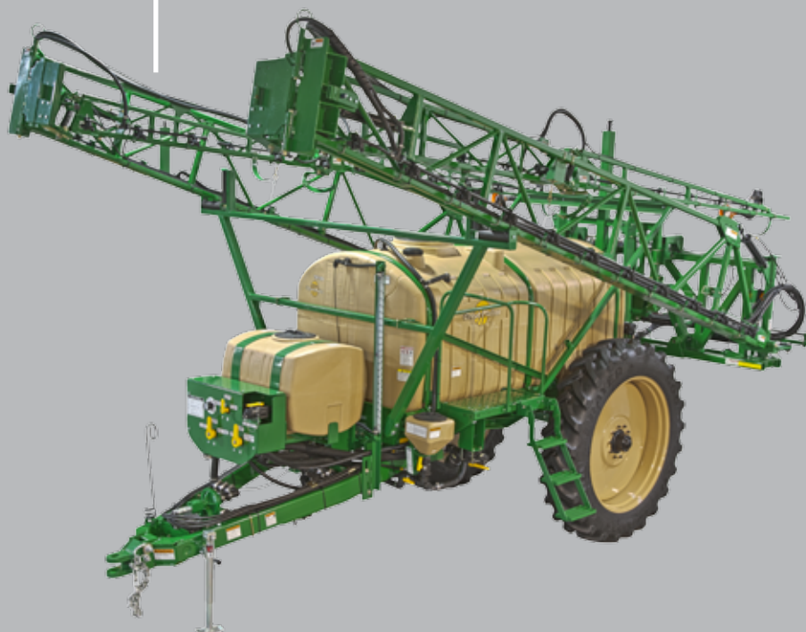
42" CUSHIONED ELEVATOR - Elevator holds boom tighter, eliminating the excess movement associated with parallel linkage.
