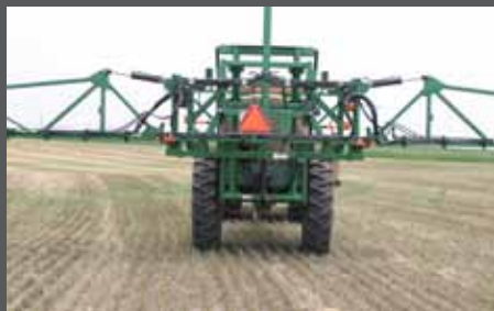
42" CUSHIONED ELEVATOR - Elevator holds boom tighter, eliminating the excess movement associated with parallel linkage.
