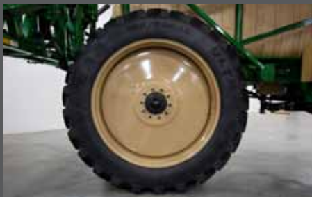
14.9x46 RADIAL TIRES - Provide maximum flotation and low compaction in the field.
