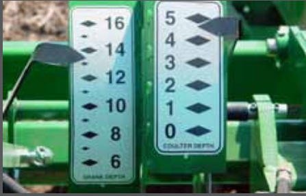
INDEPENDENT DEPTH ADJUSTMENT - Large scales show depths for shanks and coulters separately.
