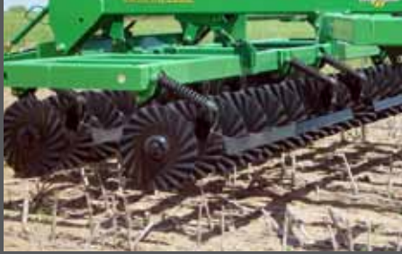
20" COULTER BLADES - Turbo Coulters size residue loosen soil without making density layers.
