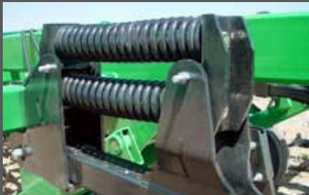
3,000 RESET TRIP SHANK - Stays at working depth in severe conditions.
