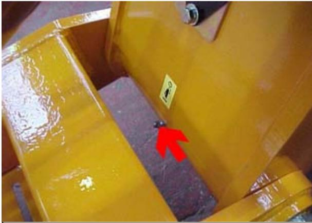
Fig. 5.14: Drawbar Pivot Grease Points
