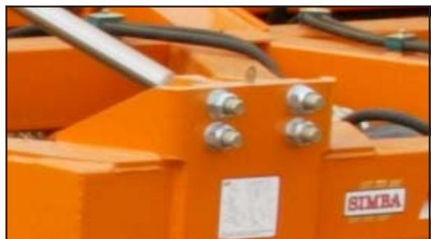
Fig. 5.05: Wing Pitch Adjustment - Solo 600
