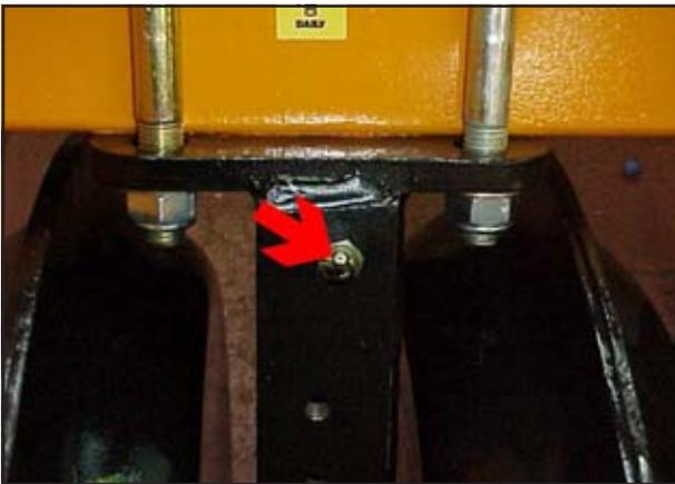
Fig. 5.08: DD Roll Grease Points
