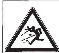
Parts may fly off during operation. Keep a safe distance away from the machine!
