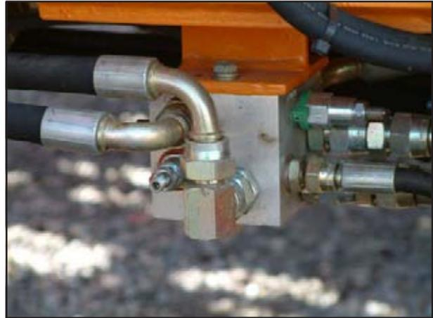
Fig. 5.06: Pro-Lift Tine Hydraulic Manifold
