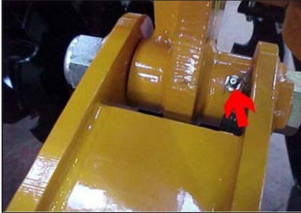
Fig. 5.12: Roll Pivot Grease Points
